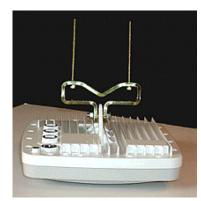
4. Place the other mounting bracket section on the two bracket mounting screws and loosely secure them with the bolts supplied. These bolts are used later to mount the radio unit to a pole (as shown in the second figure below).
